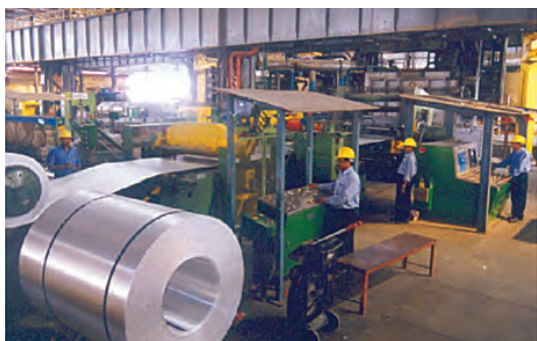
Fig. 6.6: Strip casting mill at smelter of NALCO
