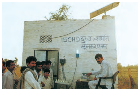
Fig. 5.11: Solar operated electronic milk testing equipment
