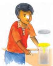
Rain Gauge: Measures the amount of rainfall
